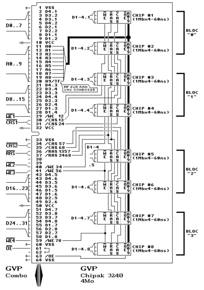
On the other hand, the 4 separate write signals /WE1, /WE2, /WE3, /WE4 still remain, although there is only one common /WE on a "regular" SIMM. This is why the SIMM 72 pins needs to be hacked.
